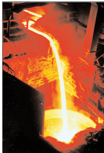
Tapping of Hot Metal at SAIL Plant
