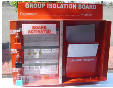
Activated Group Isolation Box with Personal Locks of Employee & Contractor and Group Isolation Lock
