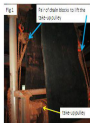
Potential Energy Isolation arrangement for belt conveyor
