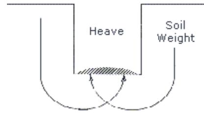
**f) BOILING** is evidenced by an upward water flow into the bottom of the cut. A high water table is one of the causes of boiling. Boiling produces a "quick" condition in the bottom of the cut, and can occur even when shoring or trench boxes are used.
