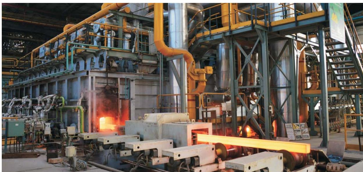
*Special Bar Mill of capacity to produce 7.5 lakh tons per annum of plain rounds in straight length and in coil form with free size rolling for customized sizes commissioned at RINL*
