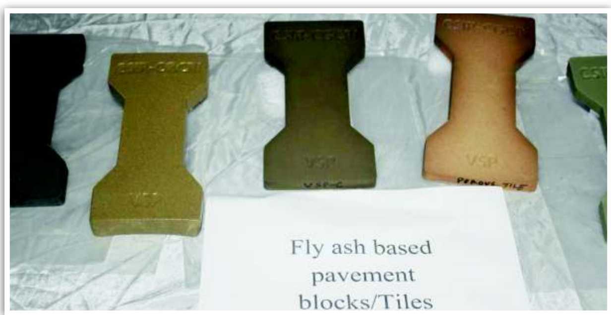
Development of pavement blocks and tiles using RINL's LD slag, BF slag, Fly ash
